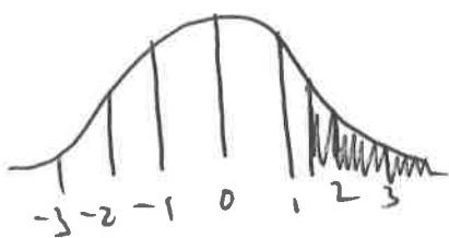
or on calculator, using 2 Prop Z Test ( $X_1 = 20$  defects on last years cars,  $n_1 = 100$  sample size cars last year,  $X_2 = 50$  defects on this years cars,  $n_2 = 350$  sample size cars this year,  $> p_2$  alt. hyp.) gives us  $z = 1.39$  and a p-value = .082.
